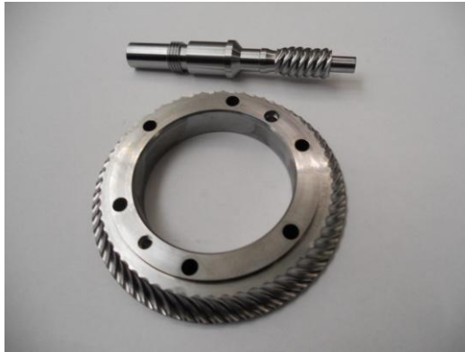
FIG.10. Wheels of rotary table gear
