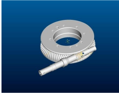
Fig.6. CAD-model of the wheels
